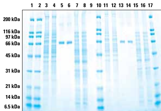
Thermo Scientific Pierce Protein Gel, 4-20%, stained with Thermo Scientific GelCode Blue Stain. Proteins were separated on 4-20% 17-well Pierce Protein Gel (Product # 84714), washed 30 minutes with water, stained for 60 minutes with GelCode Blue Stain (Product # 24592) and destained for 60 minutes (3 x 20-minute washes with laboratory tissues) with water. Lane 1, 2: MW marker; Lane 3, 4: HeLa cell lysate (1.88 µg); Lane 5, 6: Purified BSA (300 ng); Lane 7, 8: E. coli lysate (1.88 µg); Lane 9: No protein; Lane 10: MW marker; Lane 11, 12: HeLa cell lysate (0.88 µg); Lane 13, 14: Purified BSA (150 ng); Lane 15, 16: E. coli lysate (0.88 µg); and Lane 17: MW marker.
